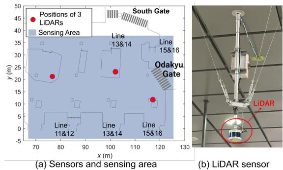
Fig.1: Sensing location, sensors, and sensor positions.
