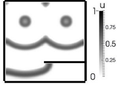
Fig.2: The numerical simulation of the two-variable Oregonator model. Waves are generated from two point sources, and shows isotropic propagation, annihilation by collision (wave-wall and wave-wave), and wall adhesion.
