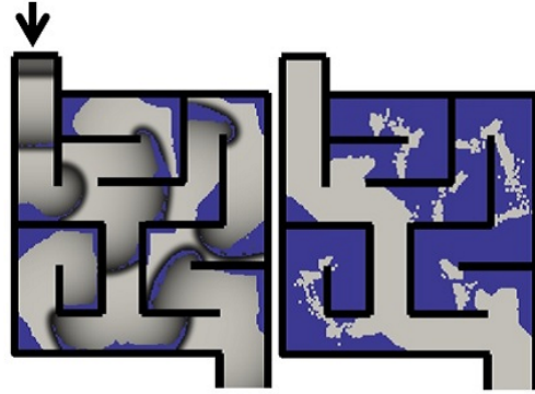
Fig.4: The numerical simulation. (Left) Waves (black bands) and the particles (blue dots) are supplied periodically. Waves propagate along the maze accompanied by particles. (Right) All of the detours are filled with the particles as time goes on.
