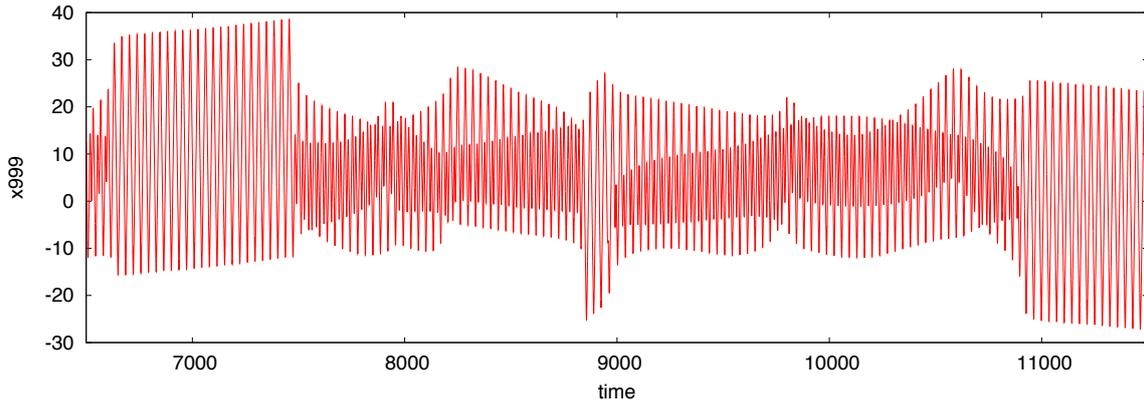
図 3:  $i = 999$  の素子の振幅変化.  $A = 5, \alpha = 3, \omega = 0.88$ .
