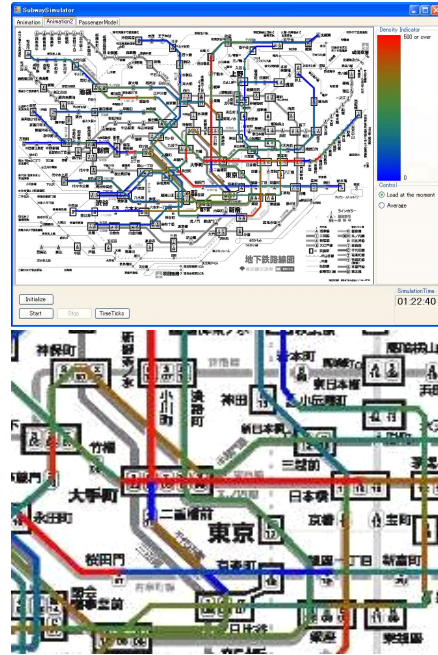
図 4: Snapshots of our simulator “KUTTY”. Left one is entire picture and right one is closeup picture around Otemachi station. In KUTTY, the high flow (low-flow) is painted in red (blue).
