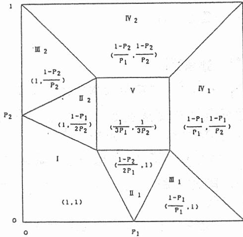
The phase diagram for traffic on two crossing roads with car densities  $p_1$  and  $p_2$ . The values in parentheses in the I ~ V phases indicate the average velocities ( $\langle V_1 \rangle$ ,  $\langle V_2 \rangle$ ) of the cars on the first and the second roads, respectively.
